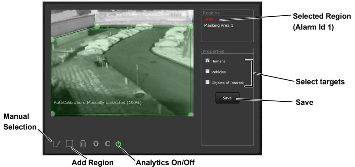
To create a detection area, click the add region icon and a new four corner area will appear on the image. Drag any of the highlighted circles to expand and define the detection area.
