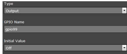
A screenshot of a configuration panel for a GPIO output. It shows three fields: 'Type' set to 'Output', 'GPIO Name' set to 'gpio99', and 'Initial Value' set to 'Off'. Each field is a dropdown menu.
