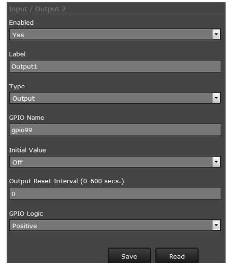
A screenshot of the 'Input / Output 2' configuration panel. It shows several settings: 'Enabled' is 'Yes', 'Label' is 'Output1', 'Type' is 'Output', 'GPIO Name' is 'gpio99', 'Initial Value' is 'Off', 'Output Reset Interval (0-600 secs.)' is '0', and 'GPIO Logic' is 'Positive'. At the bottom, there are 'Save' and 'Read' buttons.
